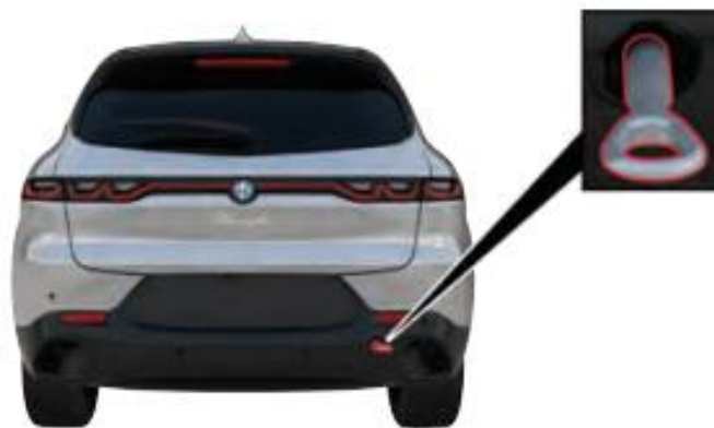
Rear Tow Eye Installed
