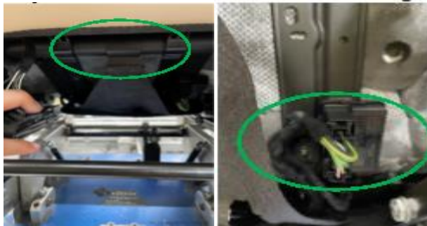
Examples of properly attached J clip (right) and harness (left)
