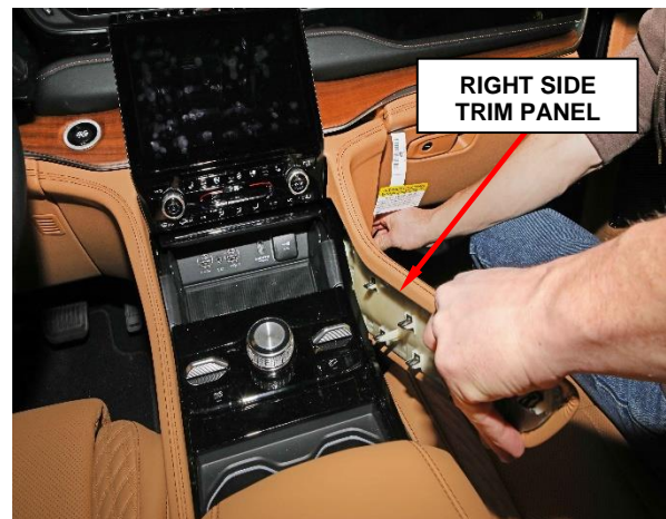
Figure 5 – Console Upper Trim
