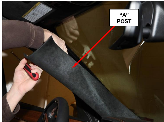
Figure 2 – “A” Post Removal
