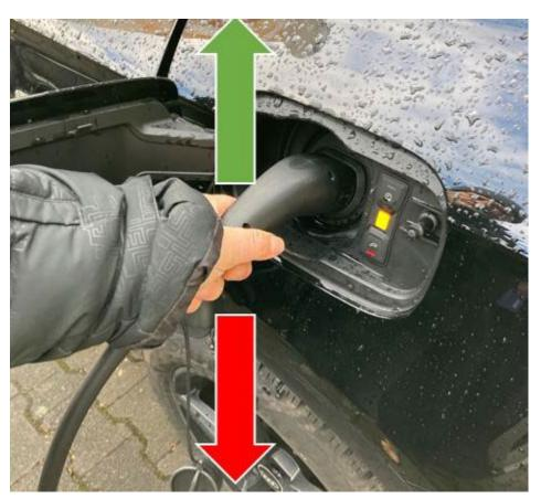
Charging connector lock not OK if pushed downwards during locking procedure (Example image from a Q5 Hybrid)
