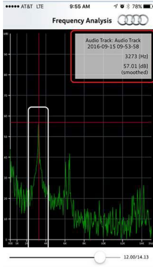
Figure 6. Typical brake squeal frequency recording.
