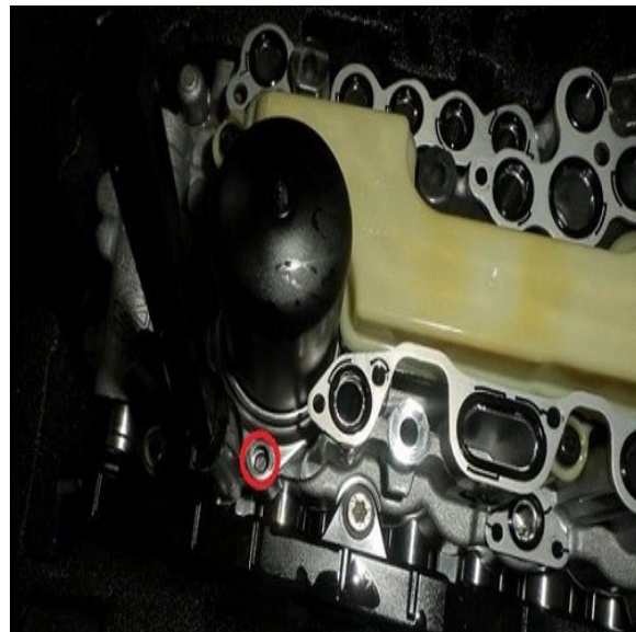
Figure 5. The bolt head is missing.
