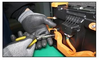
4. Replace the two voltage temperature sensor wire harnesses (VTSWH) with the new parts.
