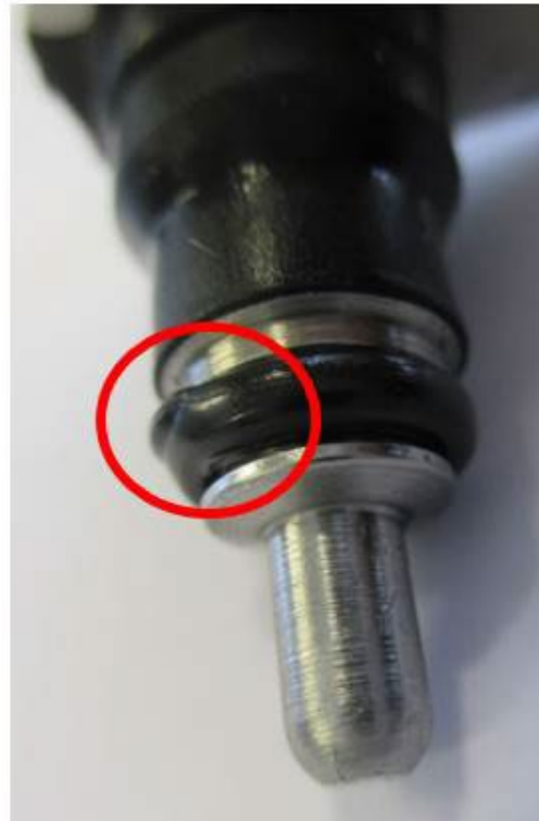
Figure 1. O-ring is pinched.
