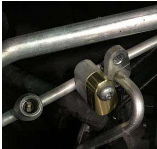
Figure 4a. Installation of high side rear A/C Line connection block adaptor VAS 6338/63.
