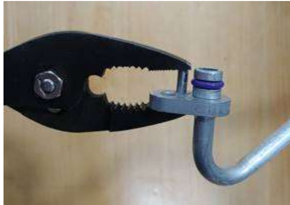
Figure 16. Installation of rear refrigerant line dowel pin.
