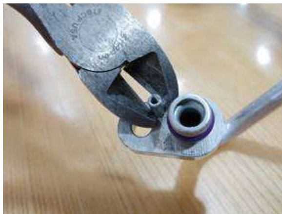
Figure 15. Removal of dowel pin.
