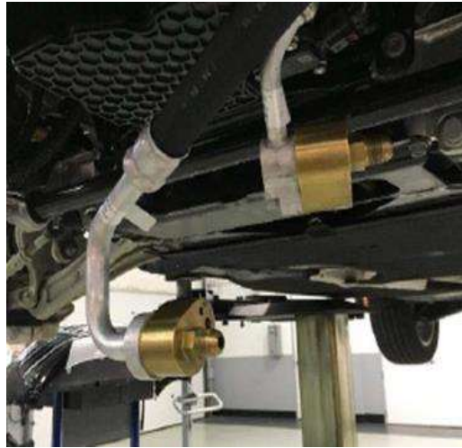
Figure 6. Installation of VAS 6338/3 and 6338/12.
