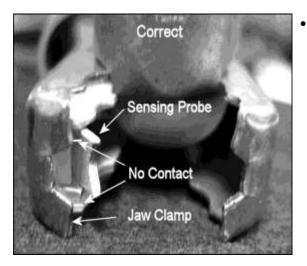
There must be no contact between the inside connection and outside jaw of clamp -arrows-.
