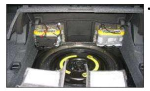
(3.2L) Test/charge AGM battery located in trunk - one
