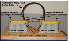
• Connect cable (Part No: 1Q0971226) to inner battery terminals.
