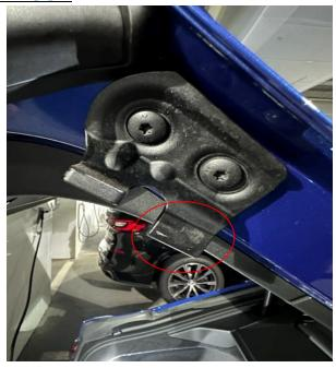
Unfavorable gap tolerance between wedging element on trunk lid and stop pad on vehicle body.
