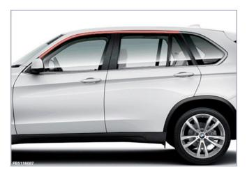
2. Clean the upper door jamb in the area shown (on the body) using silicone remover concentrate 83 12 5 A16 119 of the affected door.
