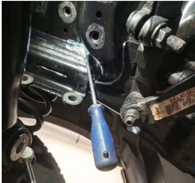
Fig. 2 Screwdriver Or Chisel Placement
