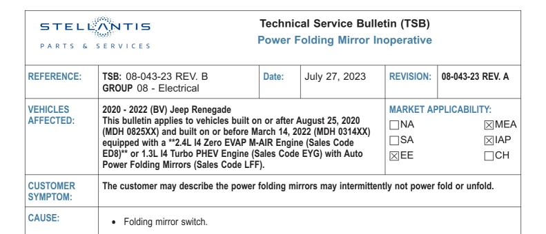
This bulletin supersedes Technical Service Bulletin (TSB) 08-043-23 REV. A, date of issue June 30, 2023, which should be removed from your files. All revisions are highlighted with \*\*asterisks\*\* and include additional engine.
