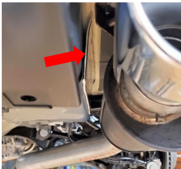
Fig. 2 Heat Shield Installed
