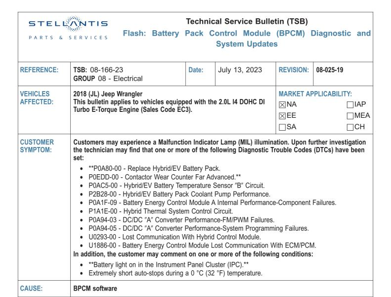
This bulletin supersedes Technical Service Bulletin (TSB) 08-025-19, date of issue March 16, 2019, which should be removed from your files. All revisions are highlighted with \*\*asterisks\*\* and include additional DTCs, Symptom/Condition and LOP.
