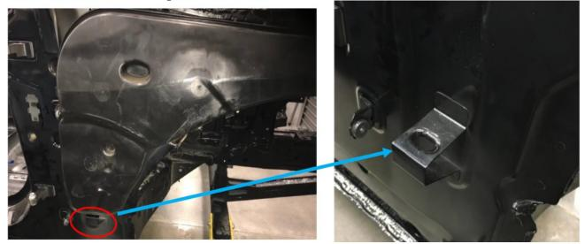
3. Wrap the lower mounting bracket with felt tape as shown.
