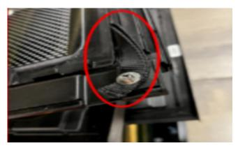
The photo shows the tether twisted. Incorrect position of tether.
