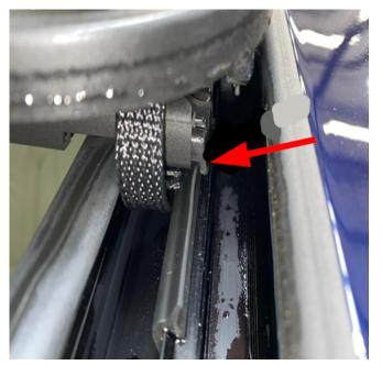
The photo shows the correct mounting orientation of the Dyko rubber seal.
