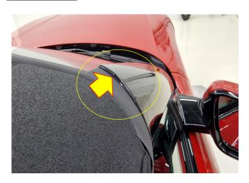
The outer A-pillar trim panel (arrow) protrudes outward (circled) towards the cowl seal.
