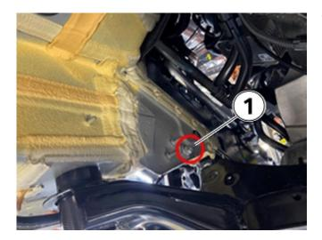
**Vehicles with the 48V starter/generator:** Replace ground nut (1) at this location on the body near the engine subframe.
