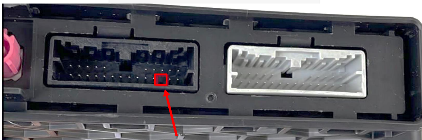
Figure 2: NOT OK ▶ pin 22 is missing.
