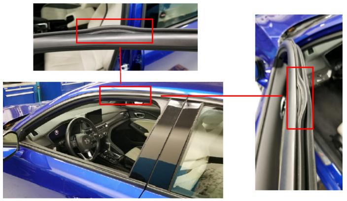
When a car comes in with this condition, you can successfully reinstall an undamaged weatherstrip back in place until permanent countermeasure parts are available.
