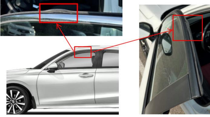
When a car comes in with this condition, you can successfully reinstall an undamaged weatherstrip back in place until permanent countermeasure parts are available.
