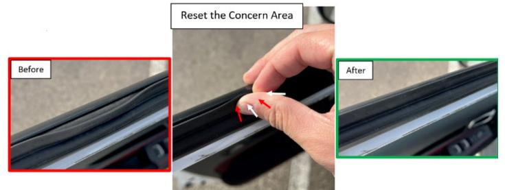
Once the weatherstrip is reattached, carefully suggest to your customer that the seal may become dislodged from the door sash if used when exiting or entering the vehicle.
