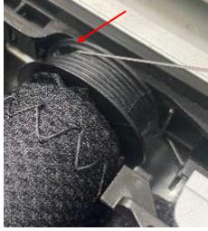
• Tension the cable on the opposite side so that the cable end and the opening for hooking the end piece are visible on the side to be repaired.
