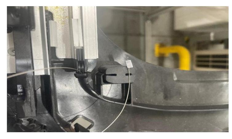
Cable end piece unhooked from the roller blind.
