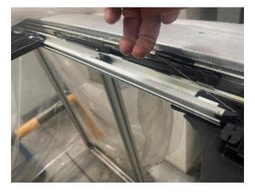
• Tension the cable on the opposite side so that the cable on the side to be repaired is free of tension.
