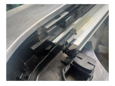
Hook the cable into the correct position of the deflecting element.
