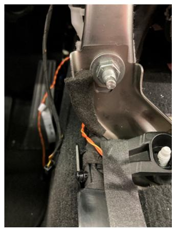
6- The knee air bag wiring should be protected from chafing at the dash support bracket.
