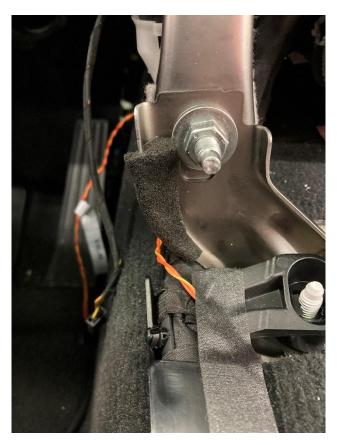
6- The knee air bag wiring should be protected from chafing at the dash support bracket.
