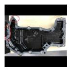
3. If there any shiny/bare surface showing poor RTV adhesion, as shown in the picture above. Take a clear close-up picture.
