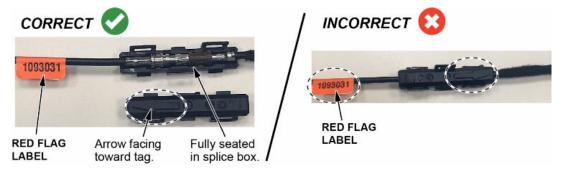
NOTE: Do not spin the splice box or the cables as this can damage the connection point.
