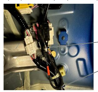
Attach the FAKRA service cable and splice box to the appropriate component harness with tape to prevent any rattles.
