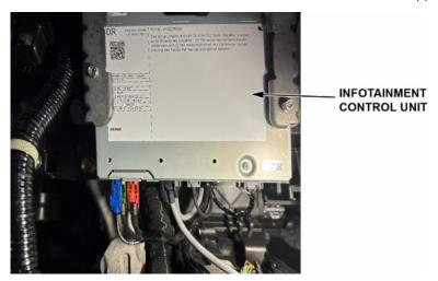
4. Install the matching color FAKRA splice repair service cables and splice boxes.
