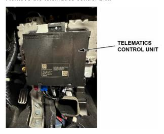
2. Disconnect the gray UG USB cable from the telematics control unit and set the unit off to the side.
