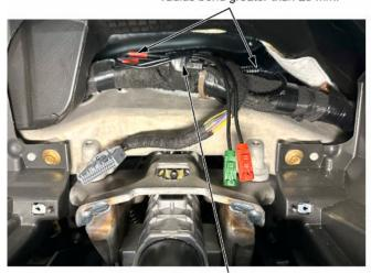
Attach the FAKRA service cables and splice boxes to the appropriate component harness with tape to prevent any rattles.
