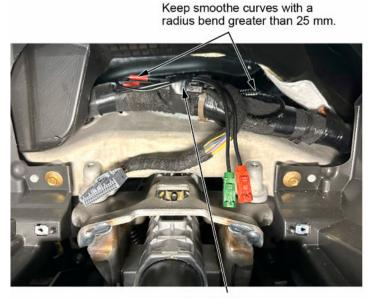
Attach the FAKRA service cables and splice boxes to the appropriate component harness with tape to prevent any rattles.
