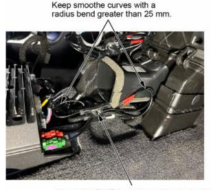
Attach the FAKRA service cables and splice boxes to the appropriate component harness with tape to prevent any rattles.
