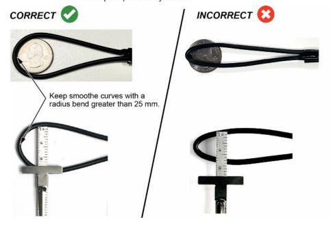
NOTE: Make sure the FAKRA splice repair service cables are not bent at the connector(s), as shown below.
