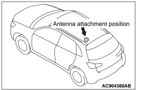
Install the antenna for radio transmission equipment only to the position shown in the figure.
