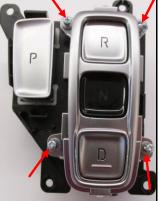
Remove 4 screws and release the tabs. Remove the cover.
