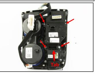
5. Release the tabs and remove the black cover. Remove 4 screws and remove the cover.
