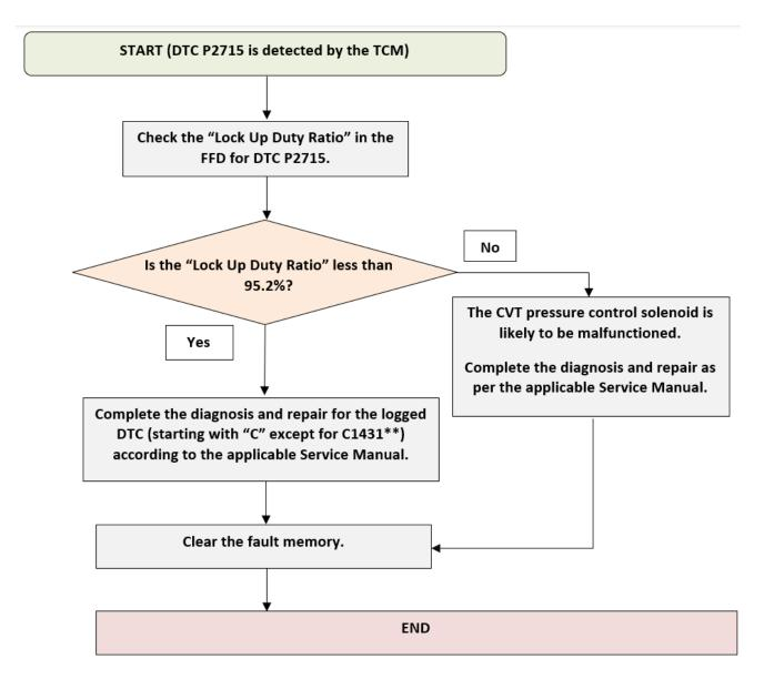
**\*\* NOTE:** Avoid following the trouble tree diagnosis for code C1431 when diagnosing P2715 misdetection. The trouble tree workflow for C1431can lead to some automatic transmission testing procedures.
