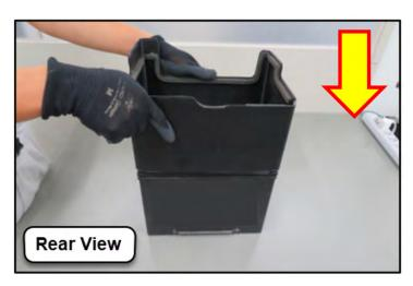
STEP 5: Assemble the ORIGINAL battery holder, NEW rear holding rod (p.n. 82161SJ000), and the ORIGINAL front holding rod as shown below. The original rod nut can be transferred to the new rear holding rod.
