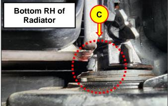
Document the coolant leaking condition at the radiator using STUI prior to radiator replacement.
