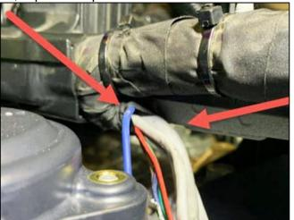
**Tucson (NX4) 2.5L – (VINs begin with KM8)** Carefully unwrap the harness protector in the area shown below. Check if the insulation has been damaged by contact with the metal bracket. If so, repair or replace the control harness.
