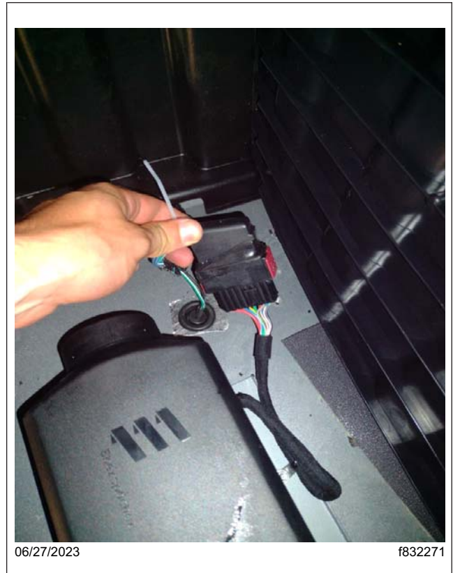
Fig. 12, Securing the Harness within the Bunk Area
