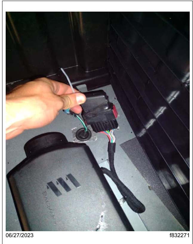
Fig. 31, Securing the Harness within the Bunk Area
