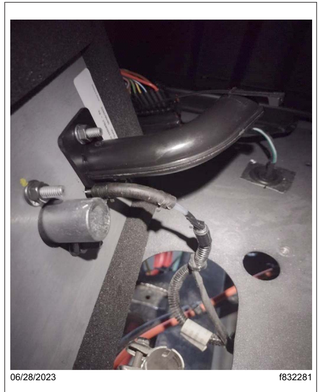
Fig. 8, Fuel Line Connected to the Heater
