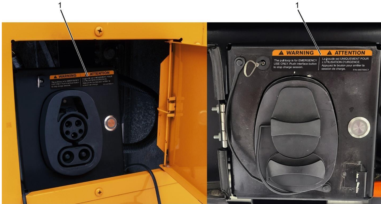
Figure 1. IC Bus Electric CE Series School Buses (“eBus”) (left) and International eMV Series Trucks (“eMV”) (right) Charging Port Locations
