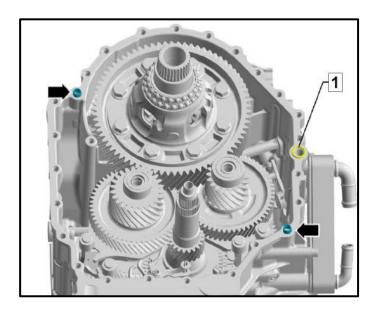
Install new o-ring <1> from the repair kit.
