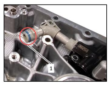
• Install new O-ring <1> from the repair kit on the changeover valve oil pipe.
