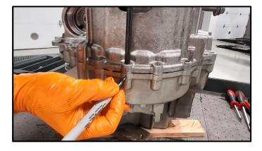
To aid in re-assembly, mark the position of both guide pins on gearbox housing with a felttip pen.
