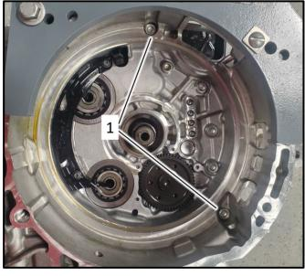
Alternate view of the two bolts <1> that are not removed at this time.
