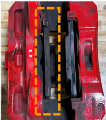
INNER PAD UNEVEN WEAR EXAMPLE - BREMBO
