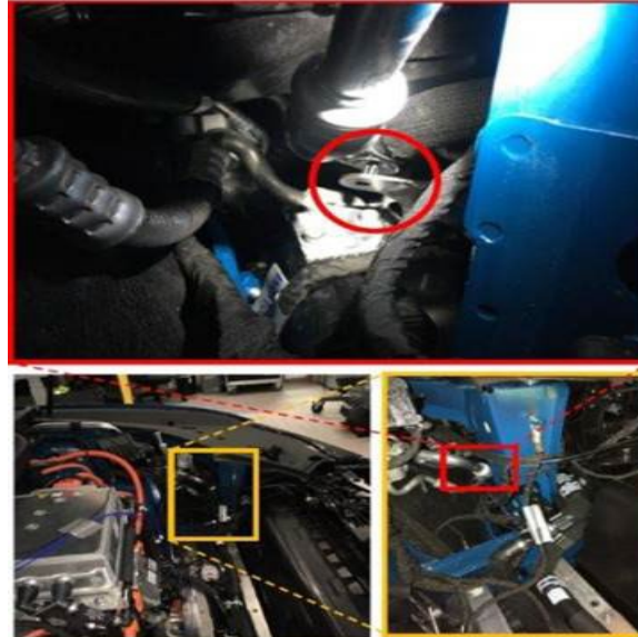
Figure 5. The area in the motor bay where contacting lines are located.
