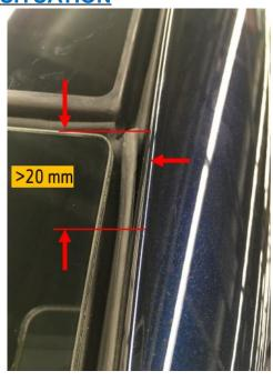
Gap between the windshield lateral seal and the A-pillar(s).
