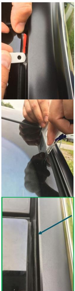
3. Cut the double sided adhesive tape to the same length as the gap on the seal. Apply the adhesive tape onto the existing adhesive tape of the windshield lateral seal. Apply from top to bottom!
