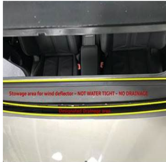
Figure 7. Areas of sunroof opening water elimination capabilities.
