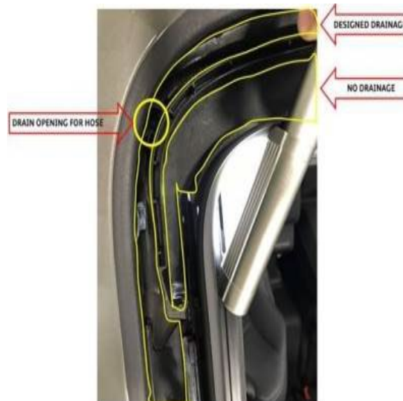
Figure 8. Sunroof water channeling diagram.
