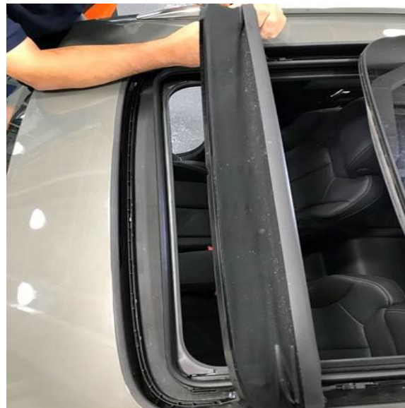
Figure 6. Front sunroof opening with the drainage exposed.
