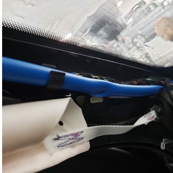
Figure 3. Sunroof drain hose pinched by the pillar trim.
