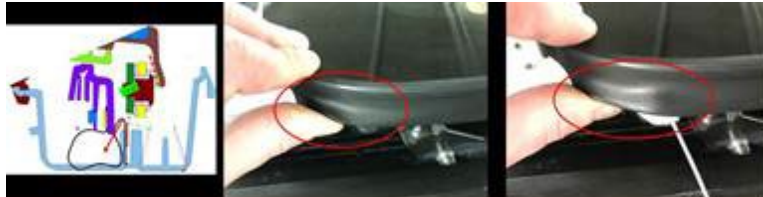
Figure 15. Area of glass panel 'skirt' where bonding agent is to be applied.
