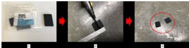
Figure 16. Preparing 2 – 10mm x 10mm pads of 251 201 525 packing.
