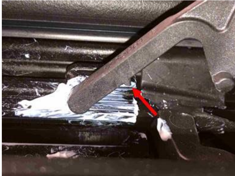
Figure 10. Tabs cast into the redesigned wind deflector.
