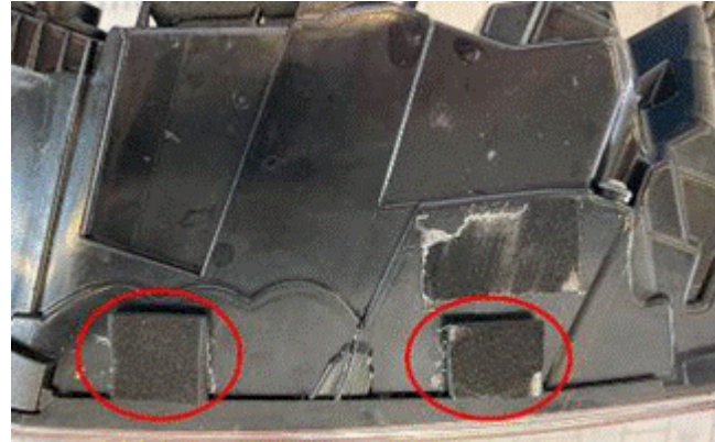
Figure 5. Foam buffer pieces reaffixed to the tail lamp housing.
