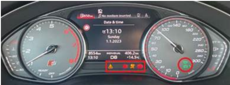
Figure 1: The warning lamps illuminated in the red rectangle are unintentional.
