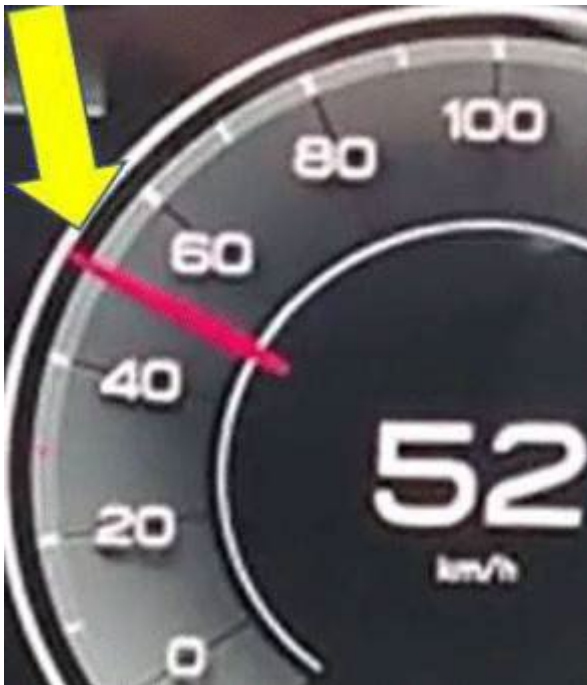
Figure 1: Red needle of the speedometer flickers while vehicle is in motion.
