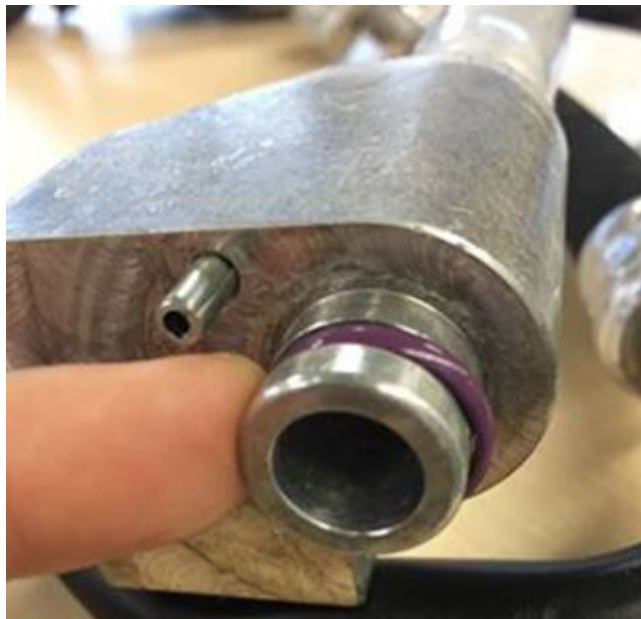
Figure 1. Damaged refrigerant line O-ring seal.
