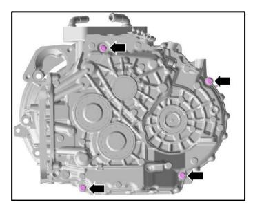
• Install new bolts <arrows> from the repair kit and torque to 20 Nm + 90°.
