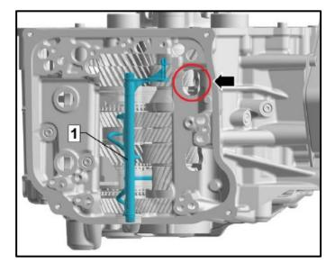
When fitting the housing sections together, you can reach through the opening <arrow> with your finger to adjust the position of the injector pipe <1> slightly.
