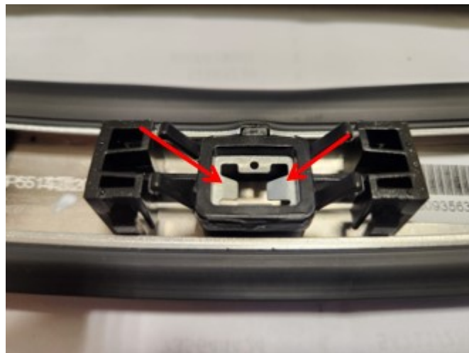
Fig. 1 Retainers Bent Out Of Position
