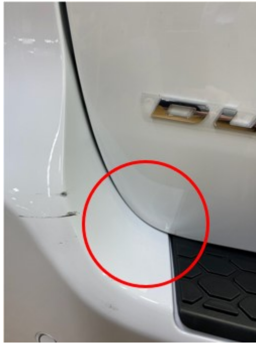
Fig. 1 Left Gap Too Tight
