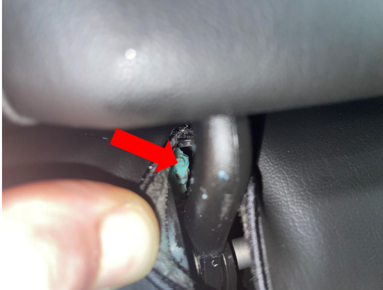
Fig. 5 Grease Added To Mechanical Pin
