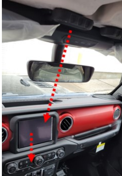
Fig. 1 Possible leaking Areas
