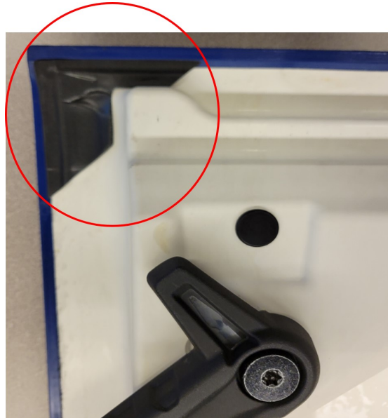
Fig. 3 Incorrectly Installed Foam
