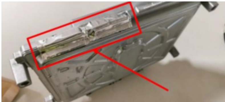
Fig. 2 Foil Tape At PCM
